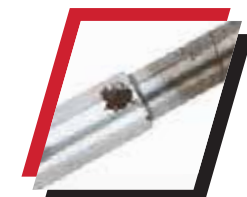
Damaged piston rod
