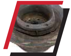
Torn strut insulator
