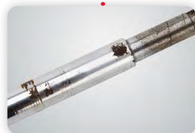
Damaged piston rod
