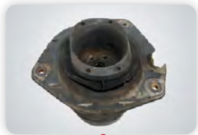
Torn Strut Insulator
